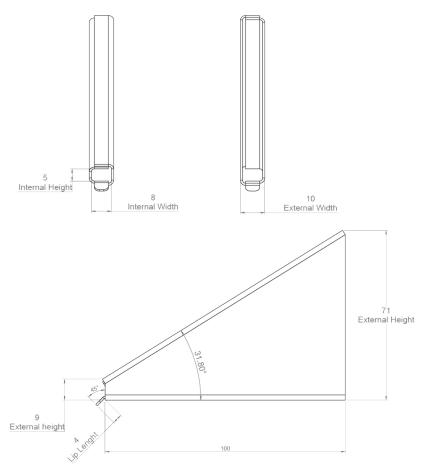
Al Non-Combustible Concealed Stainless Steel Wall Weep for use with Cavity trays directing water out of the wall cavity. Used in cavity situations in multi-storey developments where non-combustible materials are required. Stainless steel Mill finish or available with a variety of textured non-organic baked on colours preventing mortar slip.
